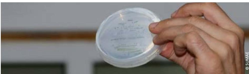
Essentially, using the streak plate technique, washed microalgae are applied as streaks using a sterile loop on agar plates in axenic conditions and kept for at least seven days to grow. Repeated streak-planting can be carried out to build up single colonies from earlier streaked agar plates and to ensure they are free from bacteria. From previously streaked agar plates, single colonies can be picked up using a loop and allowed to grow in tubes and vials (Plate 7).
