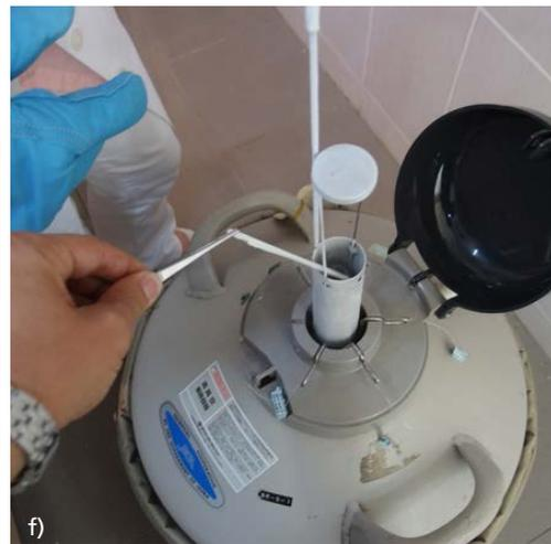
Notes: (a) collection; (b) quality determination with computer assisted sperm analysis system; (c) dilution with extender; (d) insertion into straws; (e) cooling with nitrogen vapour; (f) plunging into liquid nitrogen.
