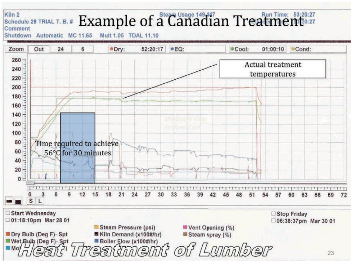
Example of a heat treatment chart for Canadian sawn wood showing that heat treatment is usually a small part of the normal operating process for an industrial kiln (highlighted area).
