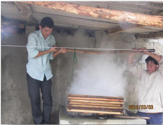
Trays of fish are being taken out of the boiler (before being moved to the drier)
