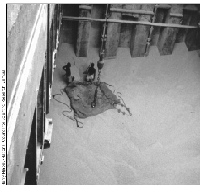
4 Mould-damaged maize in a ship's hold (typical hot spot); process of physical separation of damaged from intact kernels
