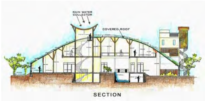
Figure 13: Double-curve roof profile
