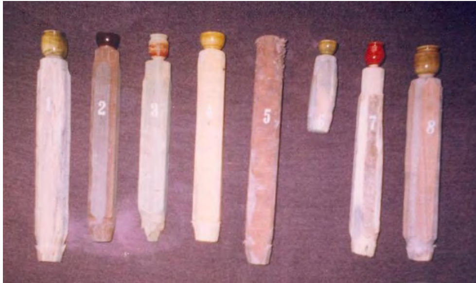
Fig.19: Trials by IWST with various alternative timbers (1.Cashew, 2.Chaplash, 3.Semul, 4.Ebony, 5.Red gum, 6.Rubber, 7.Subabul and 8Bijasal)
