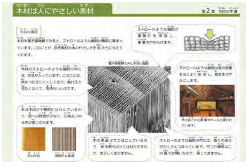
Figure 5 Teaching materials of wood structure
