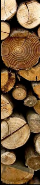
Eucalyptus log showing effects of release of stresses
