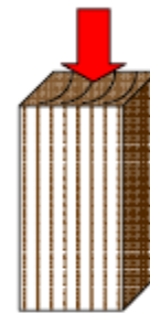
Figure 9: Compression strength parallel to grain
