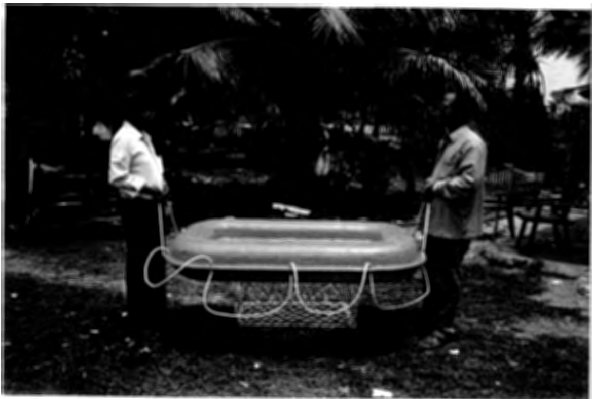
Fig. 16. Completed prototype of a 8 –10 man life float. The central bag will support two crewmembers who are old or not good swimmers. The bag will also slow down the drift of the life float when it is empty. The rope on the outside will be replaced by fixed handgrips in the next version.
