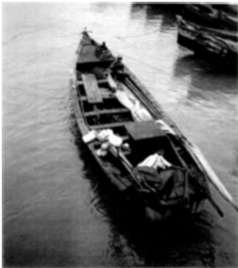
Fig.2 FRP open "Nava" with 16 hp diesel engine. Note that sail and leeboard are carried for use in case of engine breakdown
