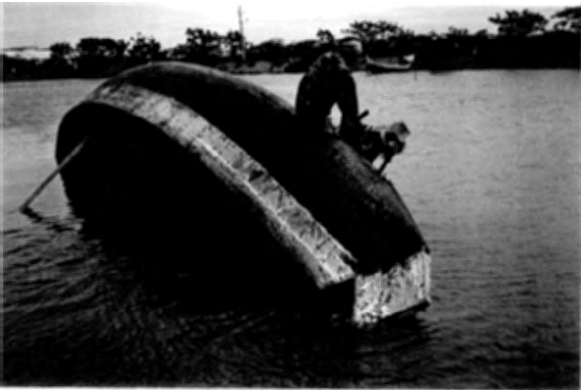
Fig. 20. The wooden Navas must regularly be turned upside down for application of hot tar to prevent attack from marine borers
