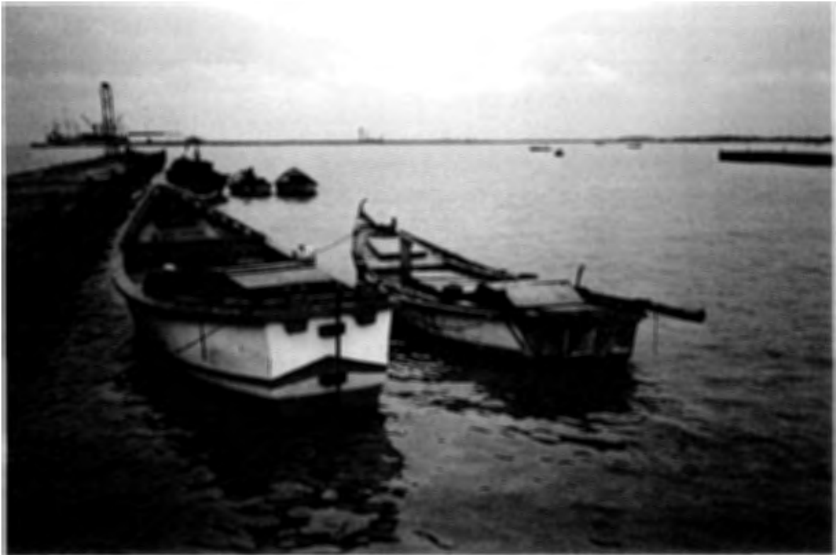
Fig. 3 Development in FRP construction. To the right is the 8.5 m beachlanding craft introduced by BOBP in 1985. To the left a recently constructed 10.7 m decked boat from Uppada, built with the same mould but expanded
