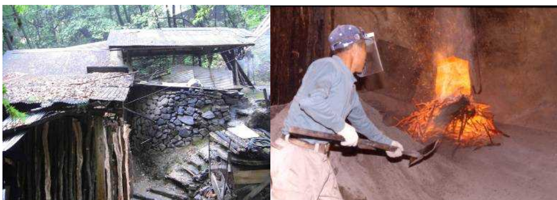
Photo 22. Binchotan charcoal kiln and removal of charcoal from kiln.
