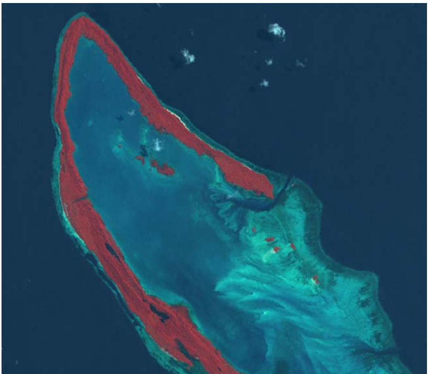
Figure 6: Landsat 7 image over the Maratua atoll displayed with a False InfraRed Colour (RGB=432) band combination; under this colour combination the vegetation becomes red because of the high reflection in the infrared range.
