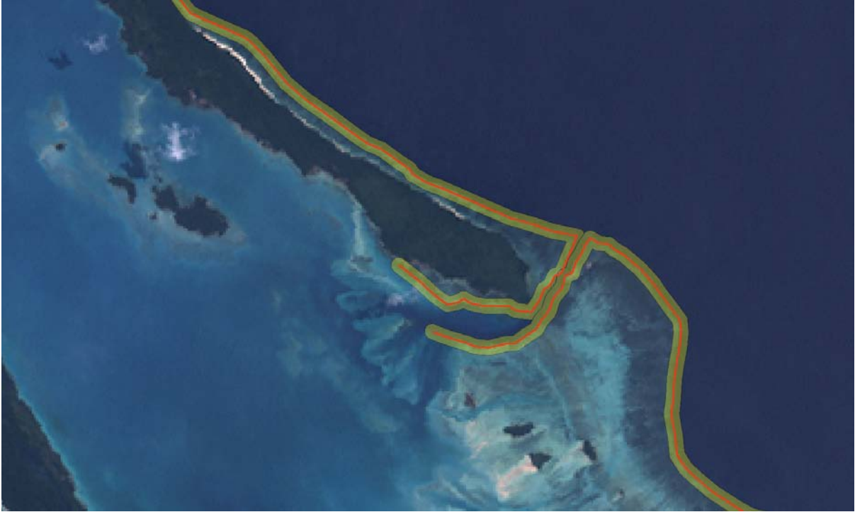
Figure 11: Example of identification and manual vectorialization of reef edges and automatic buffering on the reef edges in the Maratua atoll.
