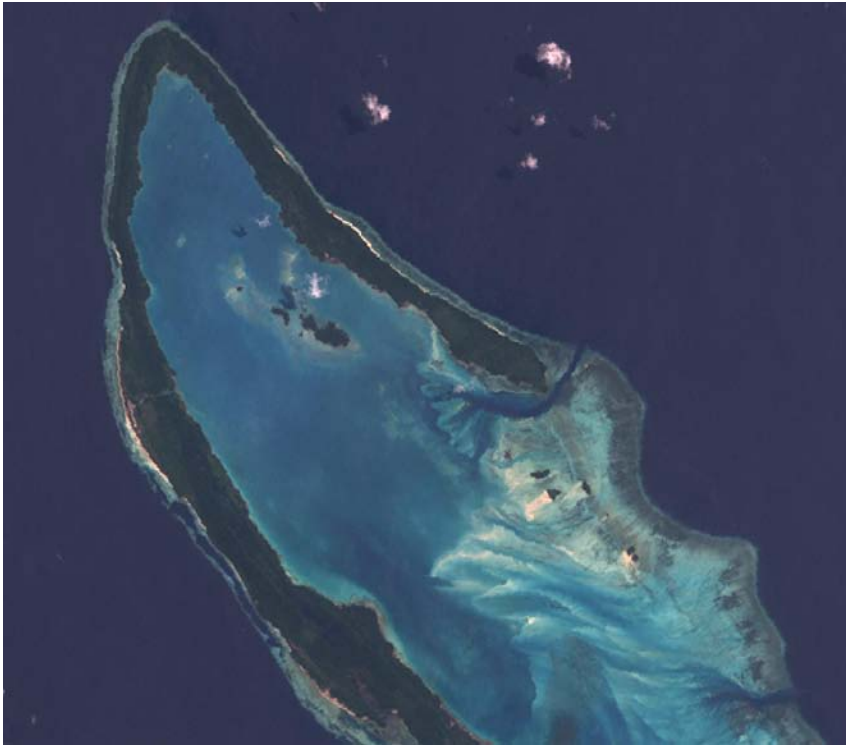
Figure 5: Landsat 7 image over the Maratua atoll displayed with a Natural Colour (RGB=321) band combination.
