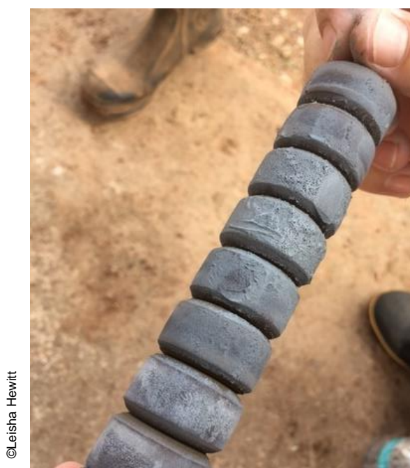
Figure 11. Build-up of residue around the recuperator sleeves
