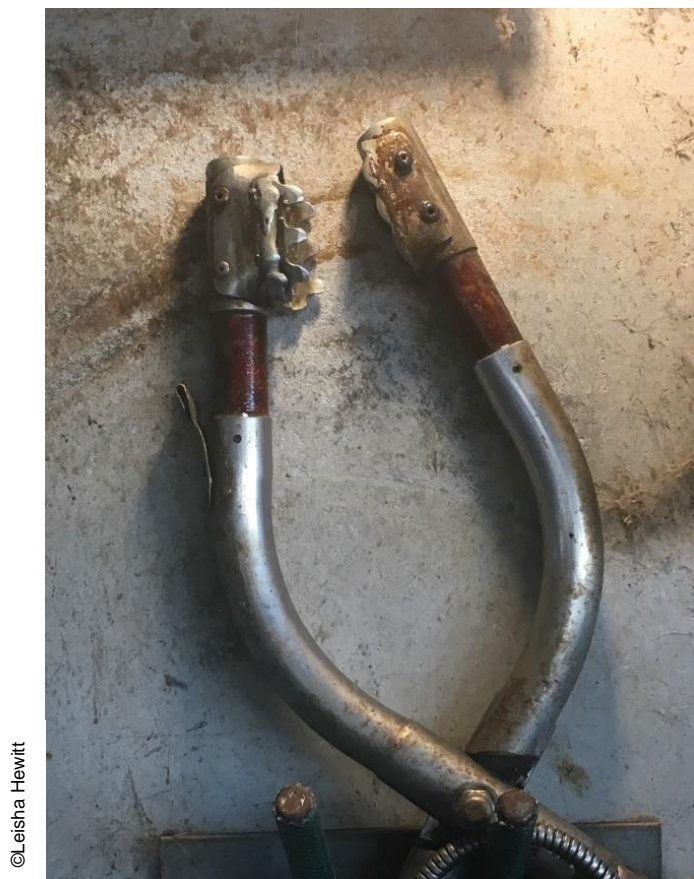
Figure 12. Worn and therefore unsuitable stunning electrodes
