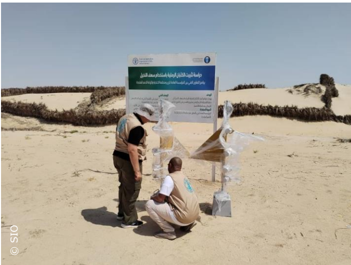
The first 2 sets of MWAC installed in Saudi Arabia.
