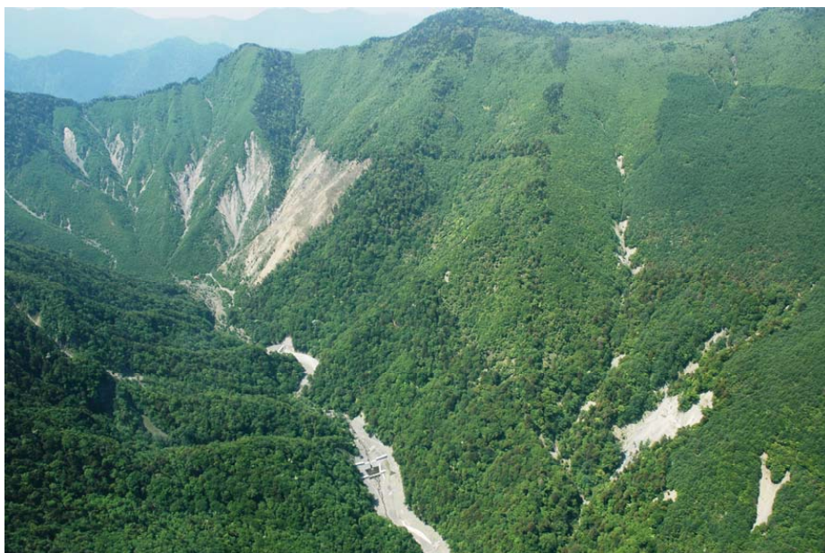
Figure 1.1. Patterns of old logging on 40-45° slopes associated with high landslide density on Kamanshi River, Yamanashi Prefecture, Southern Japanese Alps. Logging took place 5 years before the photo was taken. Notice clogging of river channel and overrun check dams
