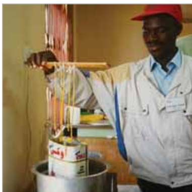
11.10 Making candles by the dipping method in Tanzania © NB
