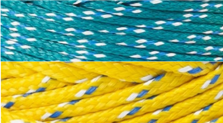
Figure 7. Colour-coded yarn identifying the manufacturer
