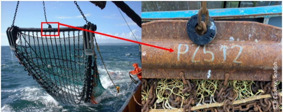
Figure 21. Marking points for beam trawl and example of a beam trawl marked with a written ID
