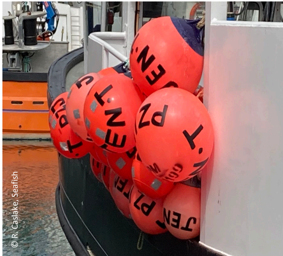
Figure 3. Surface marker buoys/floats with clear letters showing the vessel ID
