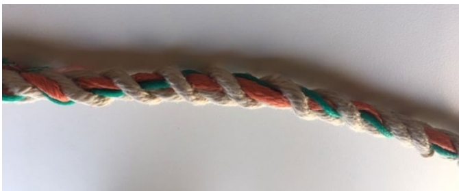
Figure 8. Splicing a rope with coloured twine to create a code
