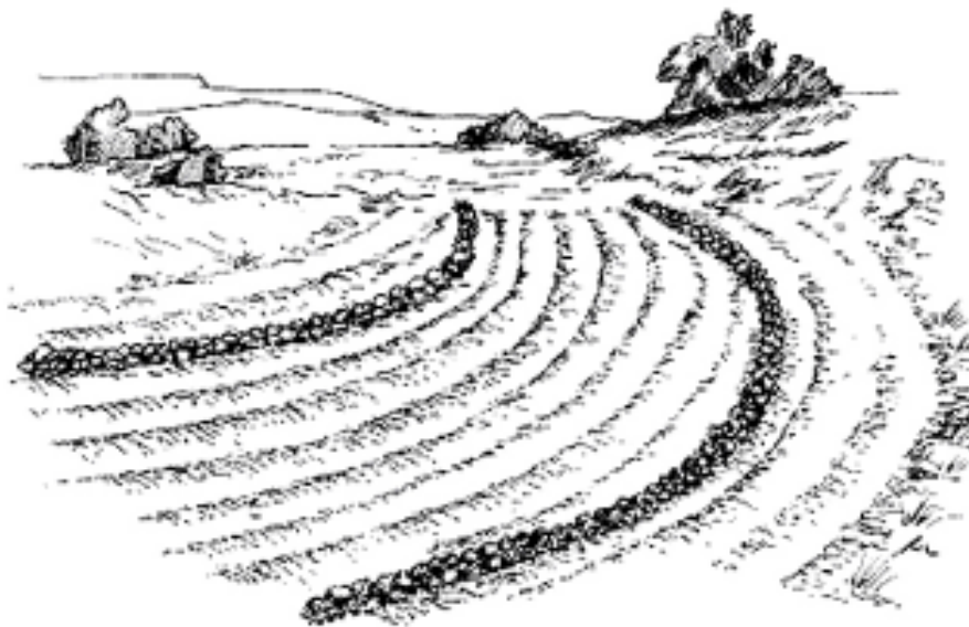
Figure 9.3. Stone lines laid along the contour slow down the runoff and encourage infiltration
