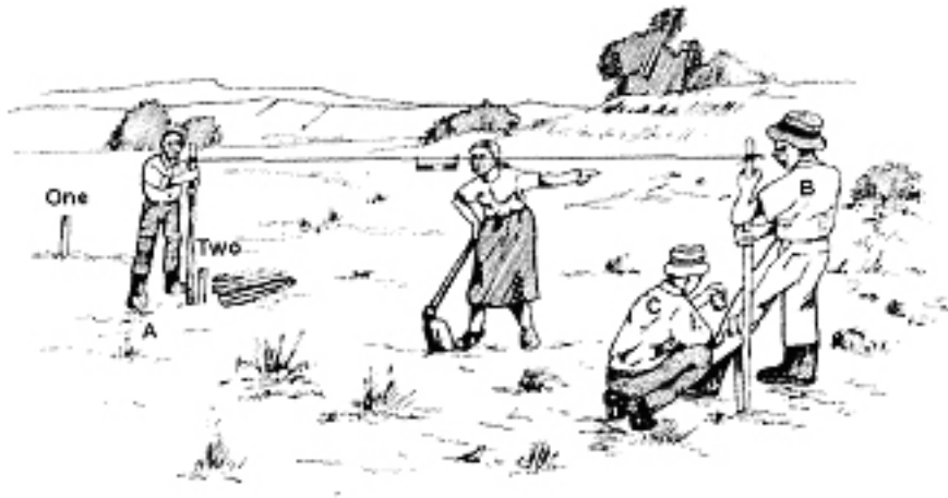
Figure 9.15. Using the line level
