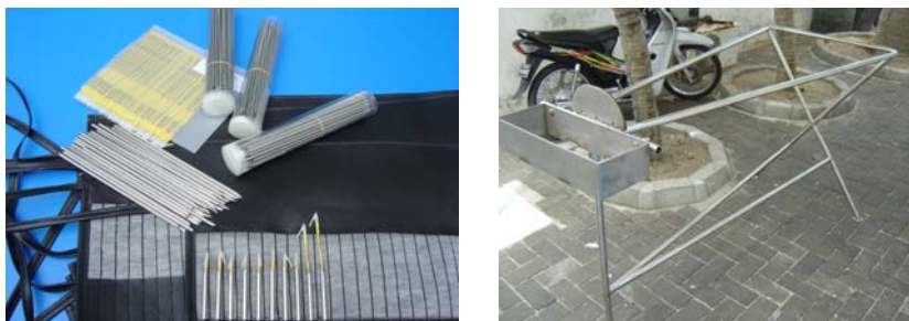
Tagging Equipment: Applicators in sleeves (right) and large cradle (frame only) for tagging large yellowfin fish (left)
