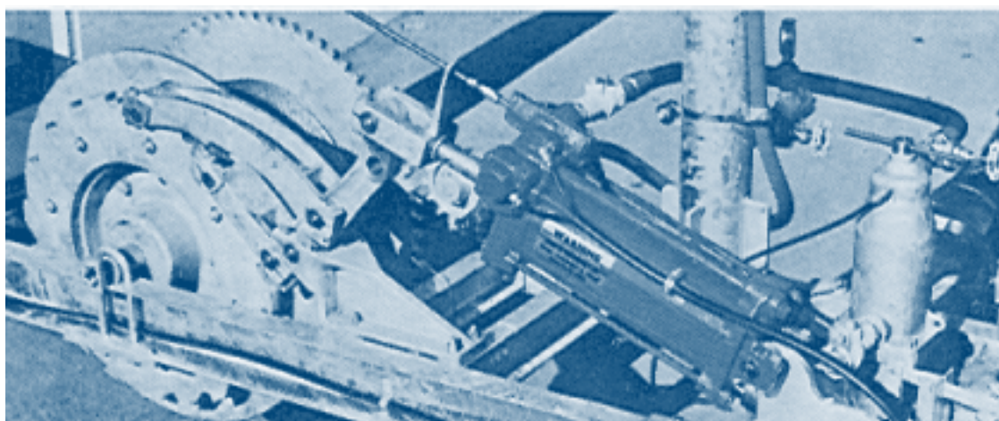
Figure 35 Hydraulic motor and winch for self-hauled cable-drawn irrigation machine (Source: FAO, 1982)
