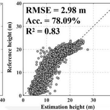
P-band DTM + DSM compensated by MLM
