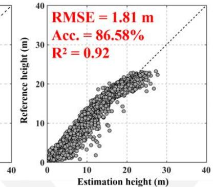
The forest height extraction based on original X-band DSM are significantly underestimated.
