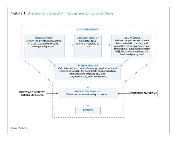
GLEAM is built on five modules reproducing the main elements of livestock supply chains: the herd module, the feed module, the manure module, the system module and the allocation module. The overall model structure is shown in Figure 1.
