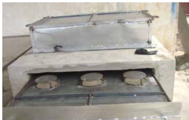
29 - Fat-collection tray with two handles inserted into the oven
