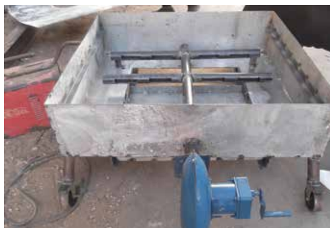
22 - Fanning forge and wheels that facilitate handling the furnace
