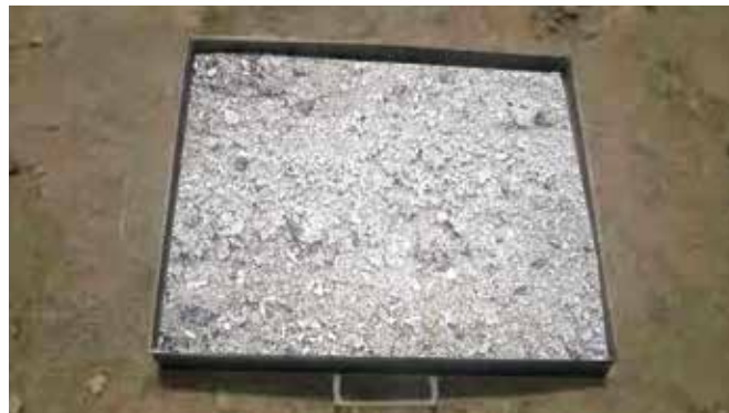
64 - Ash pan removed from the furnace to be emptied
