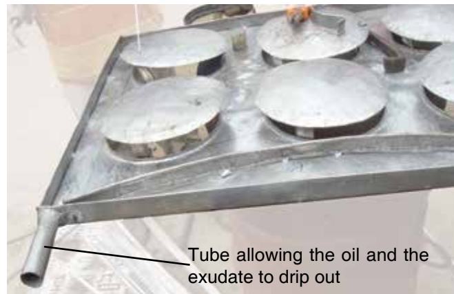
28 - Rounded iron tube soldered to the lower part of the collecting tray
