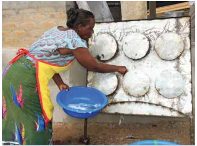
63 - Cleaning the tray of fat and exudate crust deposits
