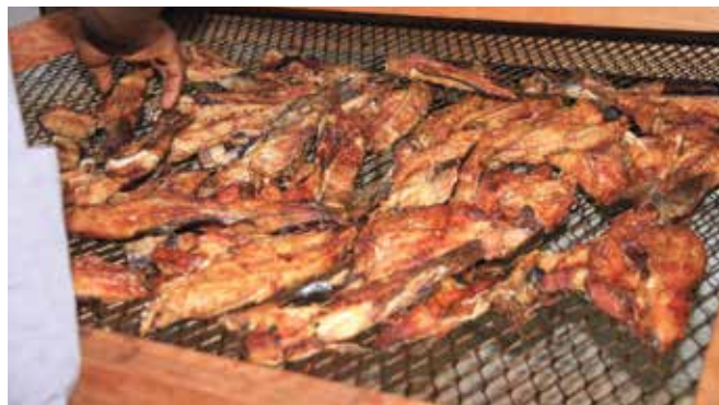
66 - Smoked fish with the FTT-Thiaroye and rack transferred from the cooking compartment to the smoking compartment
