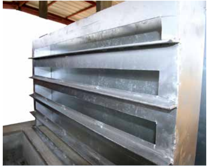
42 - Incisions/air outlets forming the fins
