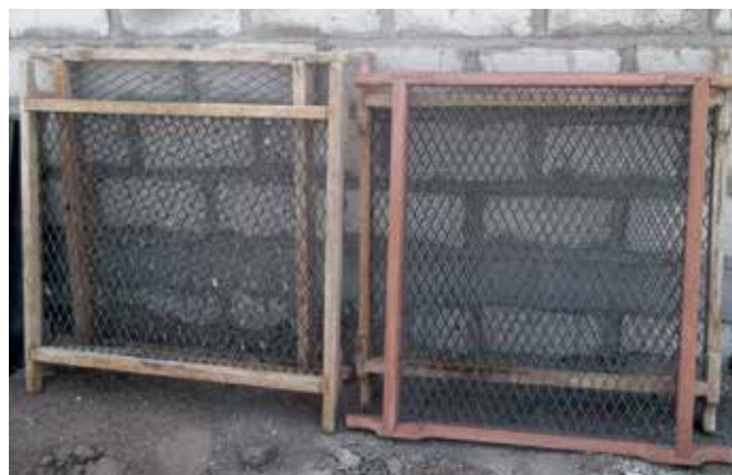
13 - Smoking racks in galvanized steel with a wooden frame
