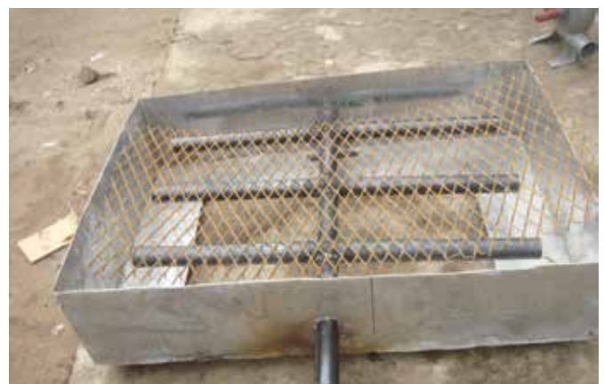
21 - Metal air tubes welded to the box and topped with a metal grid that will hold the embers
