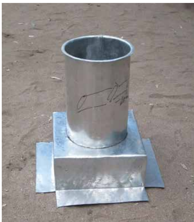
36 - The tube that will be fitted onto the gate of the smoking compartment
