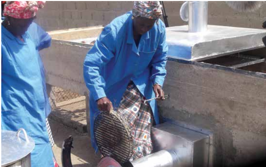
38 - Fitting the metal casing containing the filter into the indirect smoking system
