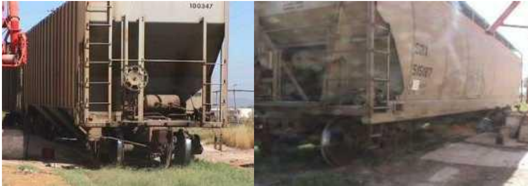
Figure 13. Soybeans and soybean meal transport by rail (left); bottom unloading by gravity (right).
