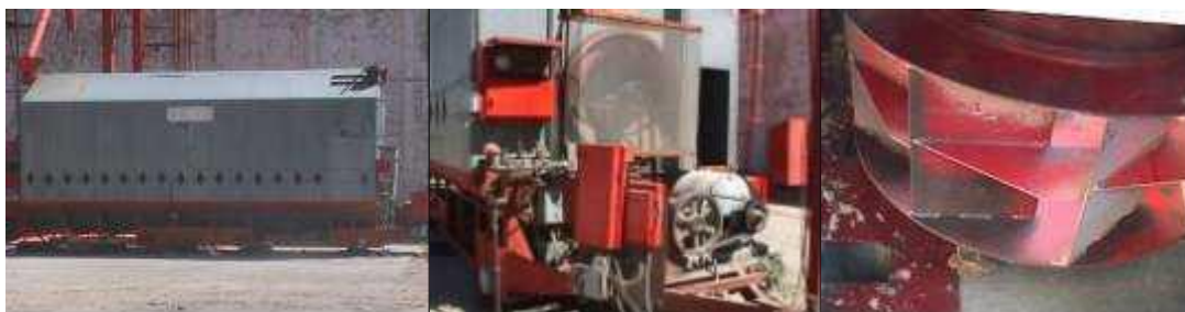
Figure 14. Grain dryer, capacity 20 tonnes/day; left: body, middle: air generator, right: ventilator.
