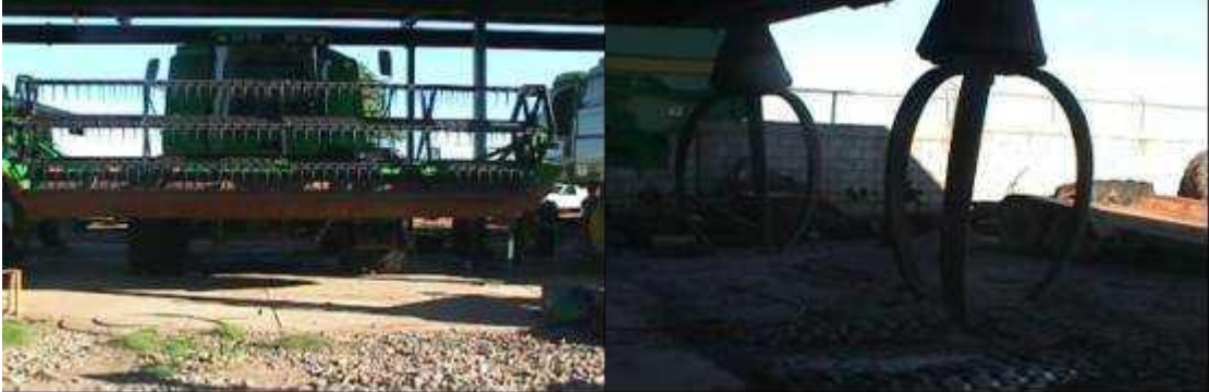
Figure 7. Modern combine for soybean harvesting, left; front view; right; back where all other parts of the plants are spread onto the field.
