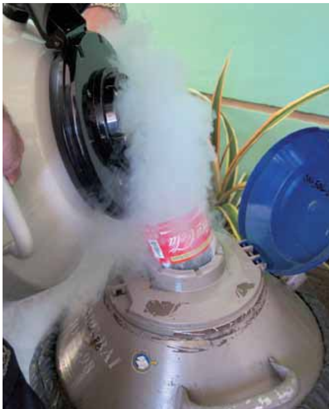
FIGURE 4.14 A dry shipper is filled with liquid nitrogen prior to field work in remote parts of the Philippines
