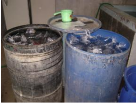
Typical ice production in Timor-Leste. Water stored in drums is used to fill plastic bags, which are closed off by tying a knot seal.
