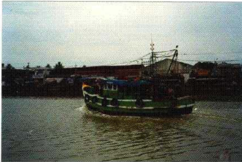
Photo 1 12 m "Sona" type shrimp trawler with 100 hp diesel engine
