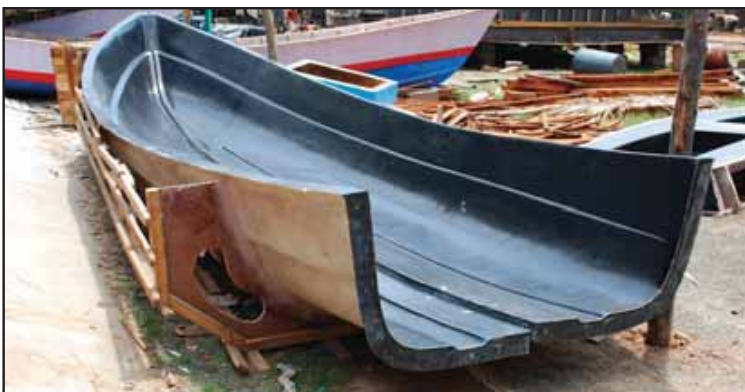
Figure 67 The completed split mould (without the transom).
