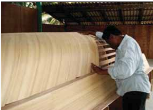
Figure 48 Diagonal strips for a curved surface.
