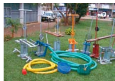
Treadle pump models (from left) - Balaji metal treadles/pulley; MG Industries/pulley; Advait, wooden treadles; Zim metal treadles/pulley; MG Industries/bicycle cog & chain; Pipeco, Mw wooden treadles/ rubber pulley; Balaji metal treadles/pivot (Photo: Z.Jere, Total Landcare Malawi & H.Phombeya, Land Resource Centre Malawi)
