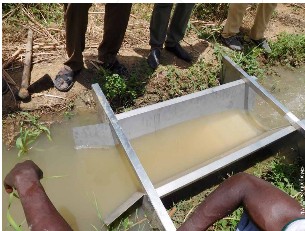
Figure 8: Portable RBC flume to measure on-farm discharge
