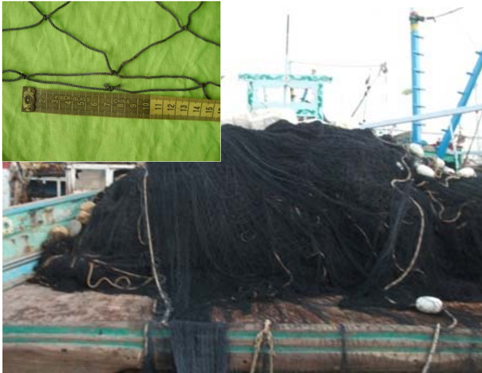
Fig. 3. Polyamide gillnet stored on board tuna fishing vessel at Karachi. Inset stretched mesh.
