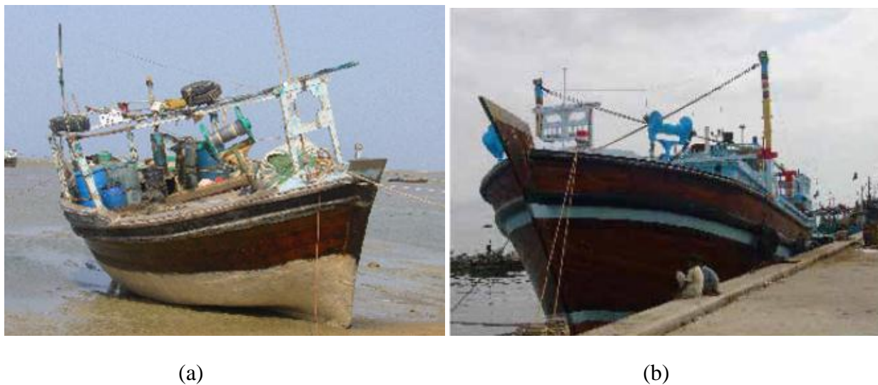
Fig. 1. Tuna fishing boats (a) Smaller Tuna Gillnetter ('hora'/'rachin') (b) Large Tuna Gillnetter
