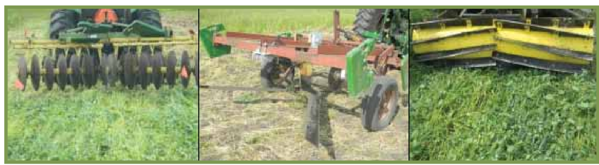
Figure 3: Implements used for management of the green manure crops at Carman (L-R): disc, wide blade cultivator (Noble blade), blade roller.
