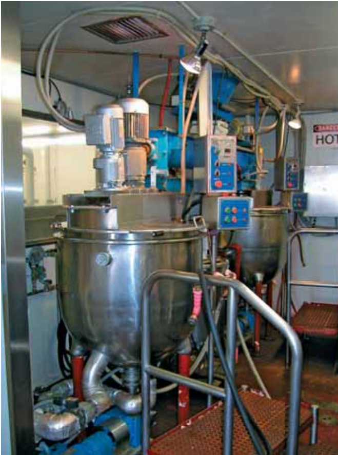
FIGURE 4 Steam-jacketed kettles for cooking the diet, each with two counter-rotating paddles to mix and stir the diet
