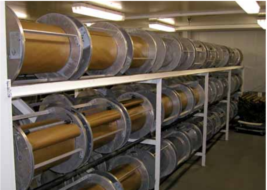
FIGURE 22 Rows of oviposition cages on slowly turning rollers (OKSIR facility, Osoyoos, Canada)
