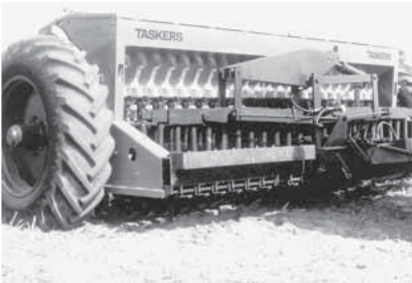
Fig. 8.6. A no-tillage drill with an 'equalizing' spring arrangement.
