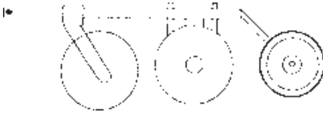
Fig. 8.9. A simple single-pivot drag-arm arrangement (slightly modified from Baumer et al. , 1994).
