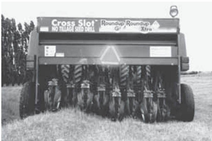
Fig. 8.8. An illustration of the extraordinary surface-following ability of a gas-over-oil opener downforce system on a no-tillage drill.
