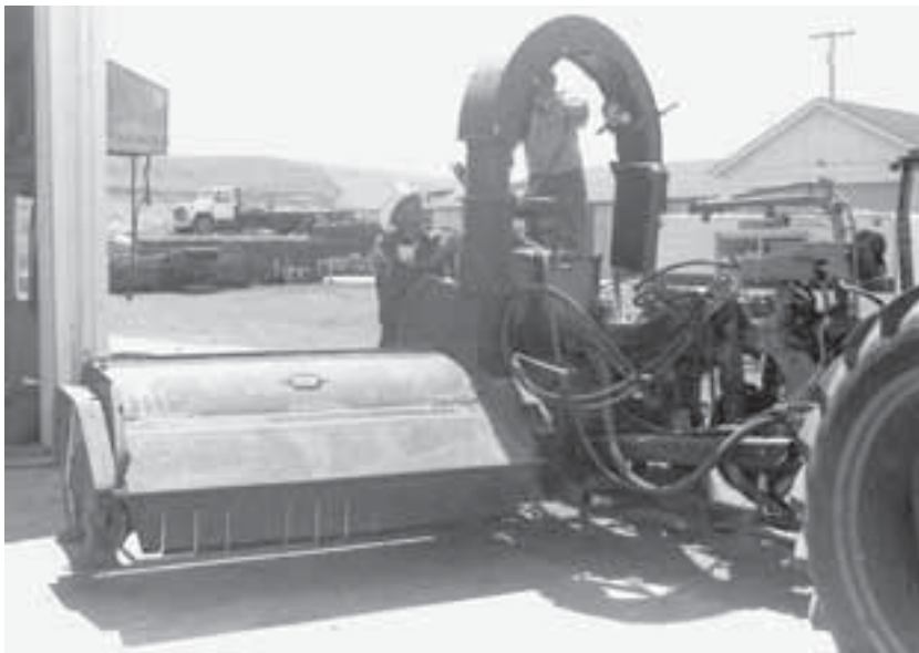
Fig. 10.12. A prototype vertical mulching machine.
