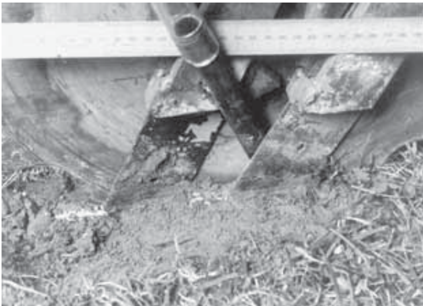
Fig. 9.4. A prototype winged opener with long and short blades for vertical separation of seed and fertilizer (from Baker and Afzal, 1986).
