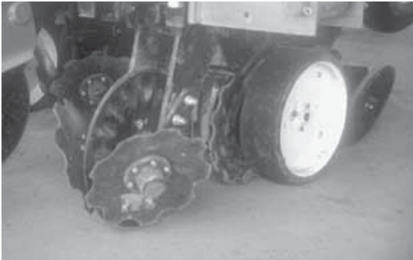
Fig. 10.11. A pair of angled, notched, disc row cleaners designed to push residues to either side of the row ahead of the opener.
