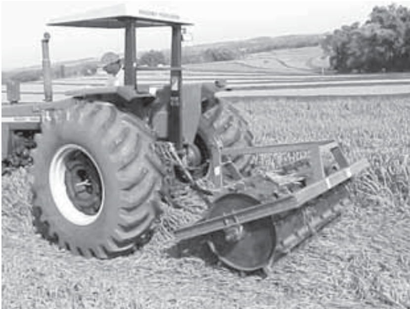
Fig. 10.6. A tractor-pulled knife roller operating in oats.
