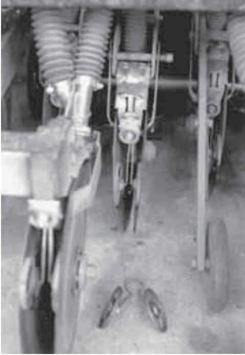
Fig. 10.19. Circular scrapers for double disc openers.
