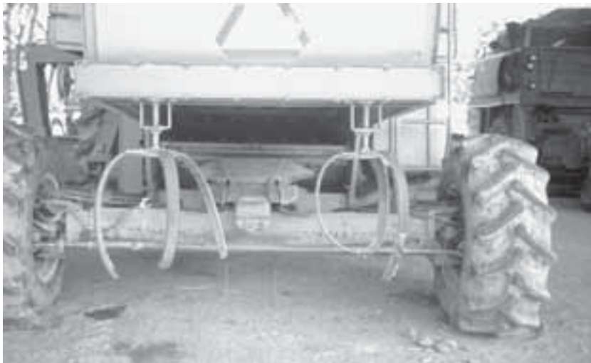
Fig. 10.3. A pair of simple beater-type straw spreaders on the rear of a combine harvester. No attempt is made to spread chaff (tailings) with such a device.
