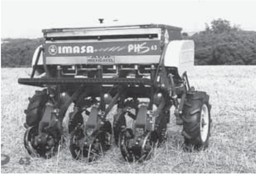
Fig. 14.10. A small tractor-drawn no-tillage drill.
