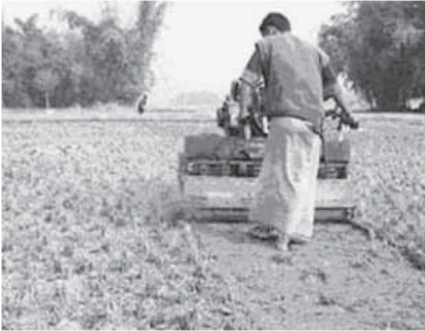
Fig. 14.20. A two-wheeled reduced-tillage machine in full-width tillage mode.
