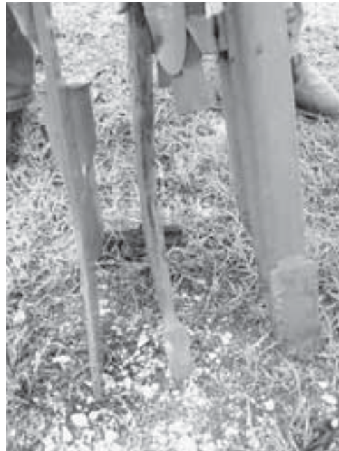
Fig. 14.4. A range of tined openers used with animal-drawn no-tillage planters. The centre opener has a groove cut into its leading edge, in which the leading disc rotates.
