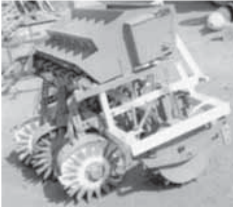
Fig. 14.16. A multi-row rolling punch planter.
