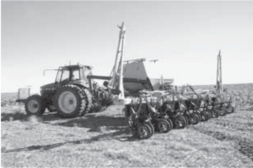
Fig. 13.3. A 4 metre rigid toolbar that is lifted clear of the ground for transport.
