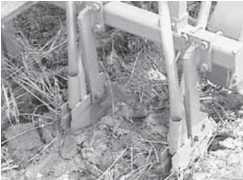
Fig. 14.13. Inverted-T openers mounted on rigid shanks attached to a square hollow toolbar. (Note that details of typical inverted-T openers can be seen in Figs 4.22, 4.23 and 4.24 – Chapter 4.)
