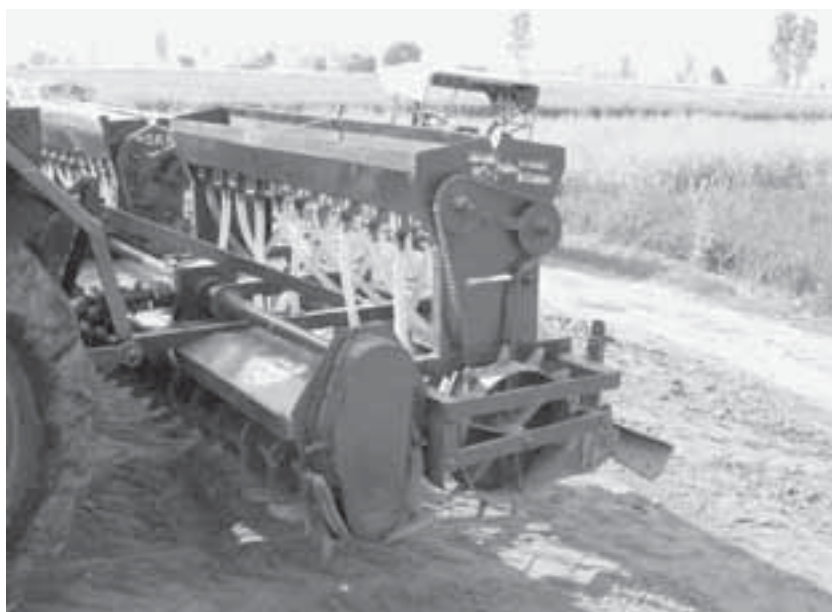
Fig. 14.15. Strip tillage drill from India.
