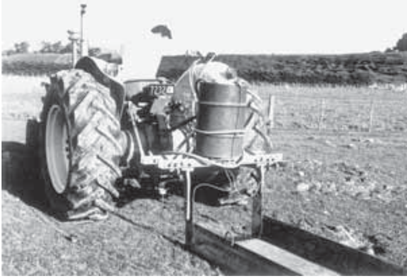
Fig. 19.1. A stirrup-shaped soil cutter with bin attached for extracting undisturbed soil blocks (from Baker, 1969a).
