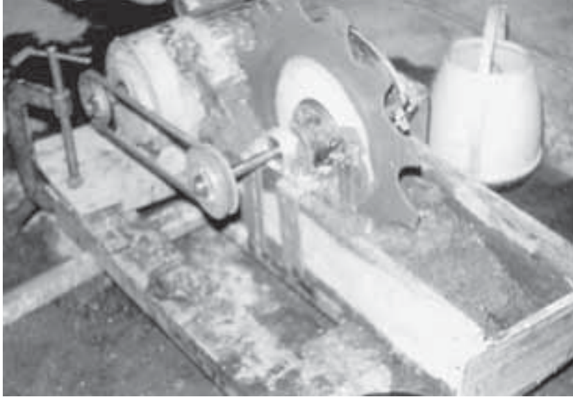
Fig. 19.11. An accelerated wear box for testing a no-tillage opener.
