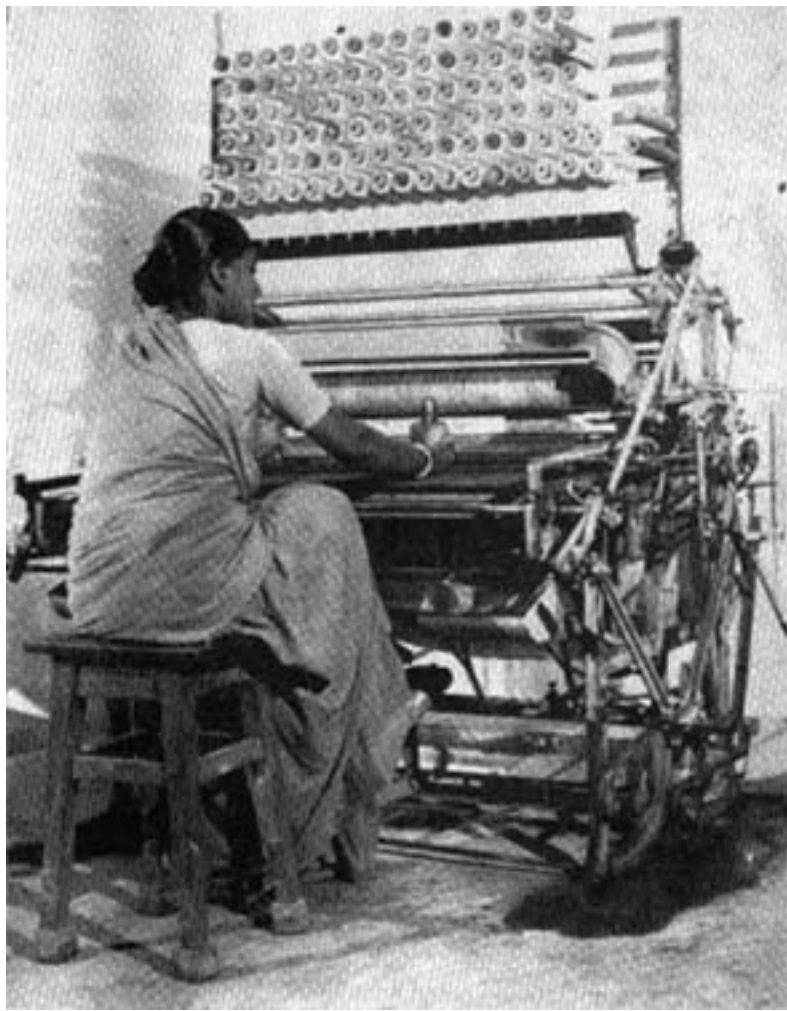
This hand-operated net making machine Was considered for introduction in fishing villages of Chingleput district to raise fisherwomen's incomes, The idea was dropped as unviable
