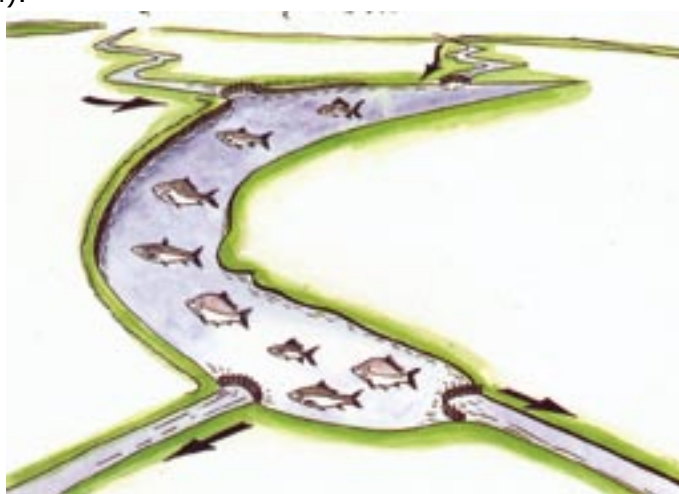
A schematic drawing of an oxbow lake to show the screening of its inlets and outlets (after OLP II, 1997b)
