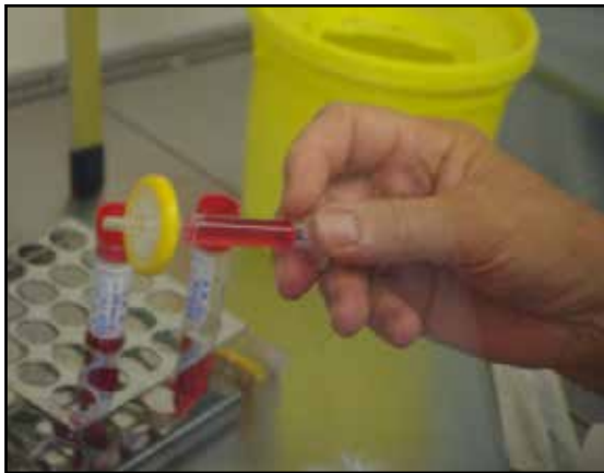
Figure 59. Filtration through 0.45 µm pore to avoid bacterial contamination
