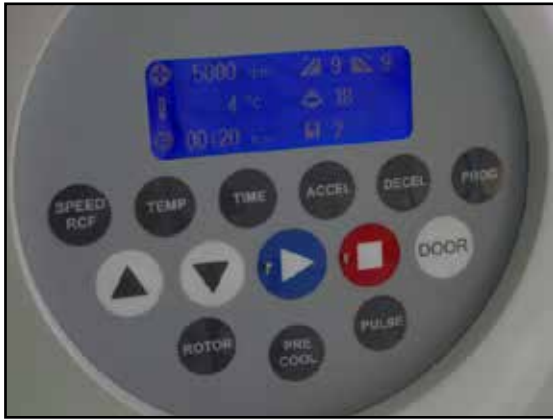
Figure 57. Material should be centrifuged in a cooling centrifuge (4°C) for 20 minutes at 5 000 pm
