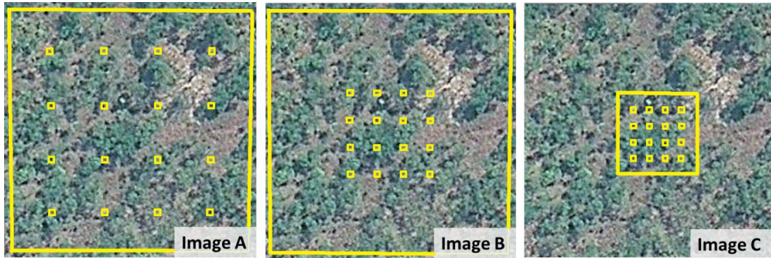
Figure 11: Examples illustrating different configurations of the Collect Earth plot layout for different spatial units. Image A: The spatial unit is a pixel block of 3 x 3. The plot layout is a bounding box of 90 m x 90 m with a margin of 15 meters between the plot border and the points and a 20 meter distance between the sampling points. Image B: The spatial unit is a pixel. The plot layout is a bounding box of 90 m x 90 m with a margin of 30 meters between the plot border and the points and a 10 meter distance between the sampling points. Image C: The spatial unit is a pixel. The plot layout is a bounding box of 30 m x 30 m with a margin of 6meters between the plot border and the points and a 6 meter distance between the sampling points. The user is encouraged to experiment with the plot layout to determine which plot layout can include the spatial unit of the reference data and compliment the project specifications. In this example images B and C have the same spatial unit, however the user might find the visual assessment is easier in image B, where the bounding box is larger.
