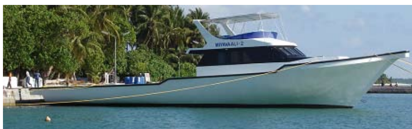
Plate A6.4 A fibreglass vessel of about 30 m.
