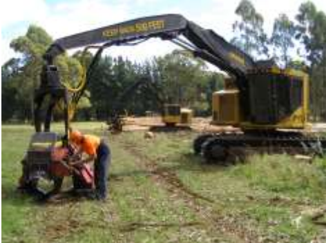
Figure 1: Minimum impact logging equipment – wide tracks and long boom with a grappling-cutting head
