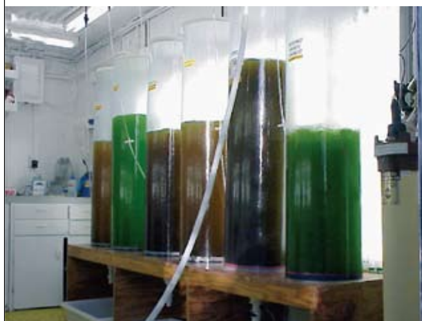
FIGURE 1 100 litre cylinders used in semi-continuous algal culture production
