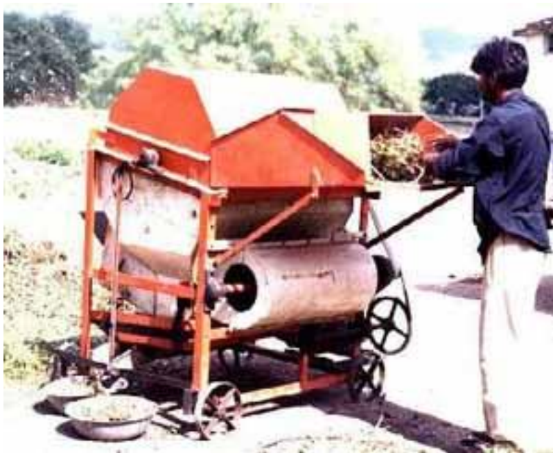
Figure 10: Groundnut stripper for stripping green vines developed by CIAE (ICAR), Bhopal.
