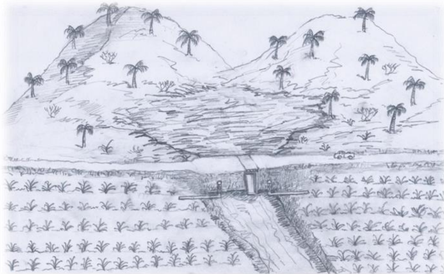
Figure 22. Sample layout of mini-dam for rainwater harvesting
