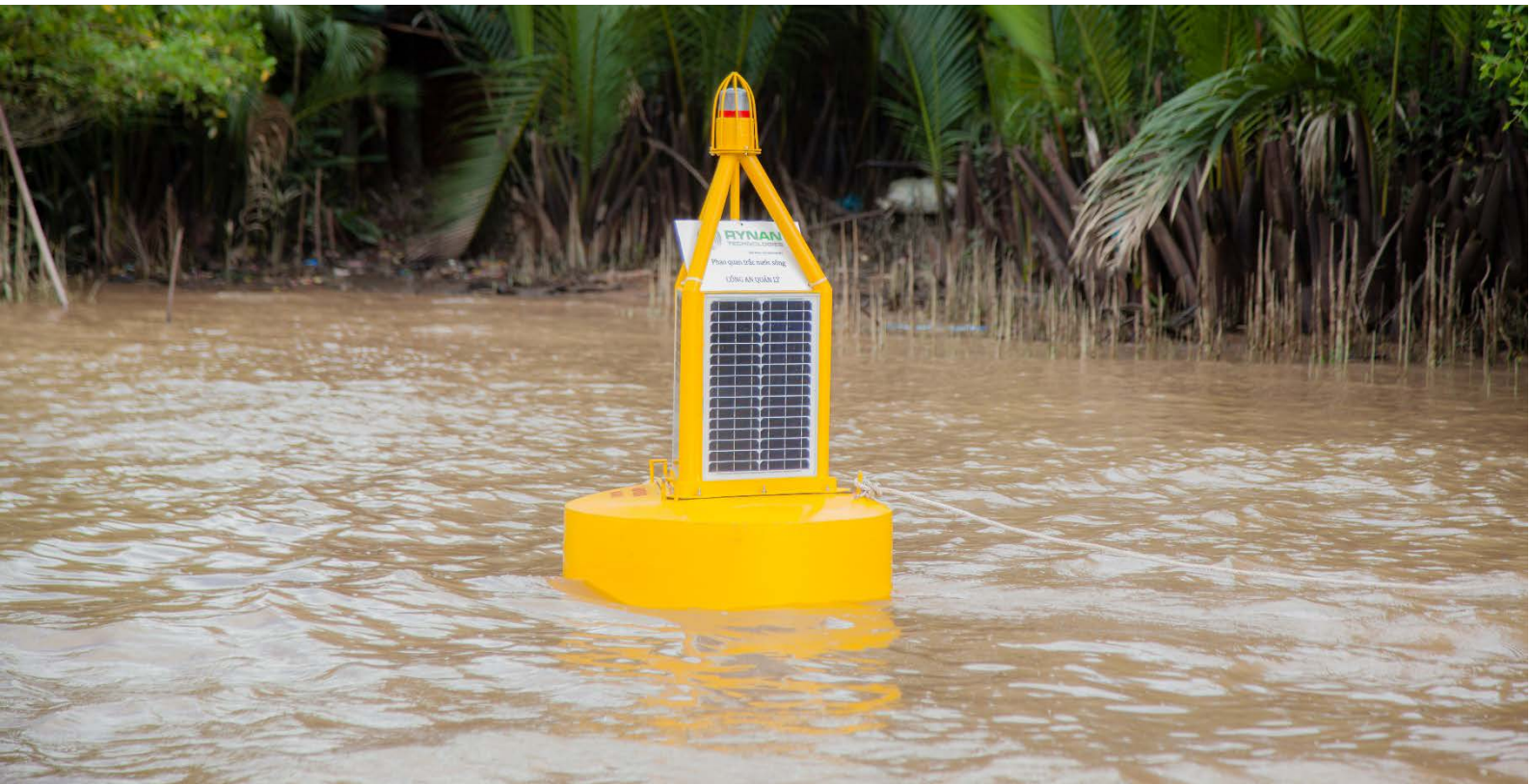
A salinity monitoring buoy in Tra Vinh province (supported by the AMD) © AMD
