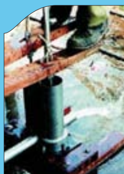
FIGURE 13. Testing pressure treadle pump by FAO-SAFR in Zimbabwe
