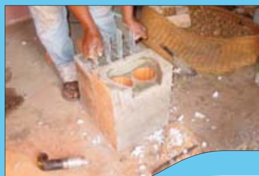
FIGURE 15. Manufacturing concrete treadle pump — FAO-W3W in Madagascar
