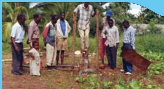
FIGURE 55. A demonstration of the concrete treadle pump - FAO-W3W in the United Republic of Tanzania
