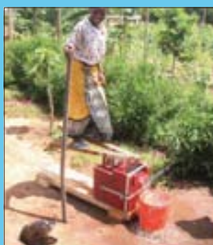
FIGURE 14. Operating the concrete treadle pump — FAO-W3W in the United Republic of Tanzania
