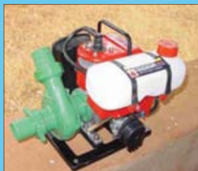
FIGURE 17. Small 1.5 HP petrol motorized pump – SPFS in Madagascar
