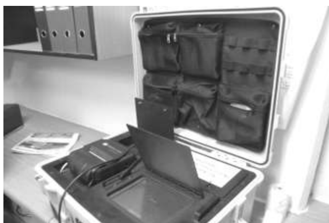
Picture 23: Portable computer and scanner used in the Livestock Identification and Trace-back System
