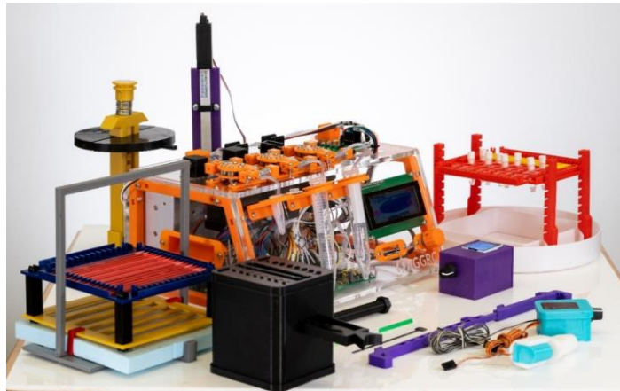
Figure 4. Examples of different open hardware devices that can be produced by using consumer-level technologies such as CAD, 3-D printing, laser cutting, microprocessors, simple electronics, and printed circuitry. Devices such as these can be used for sample processing, cryopreservation, and quality management for aquatic species, and can be made available as printer or design computer files that can be shared and modified ( www.aggrc.com ).
