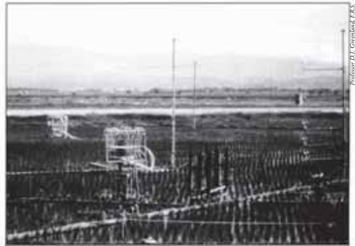
Figure 28 Measuring ammonia volatilization from nitrogen fertilizer applied to rice at the International Rice Research Institute, Los Baños, Philippines.
